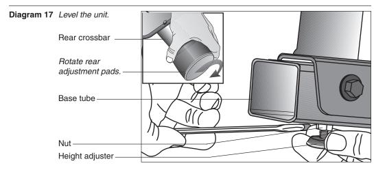
21. Level the unit. Diagram 17. To keep the unit stable, the EFX has adjustable rear pads and, at the front of the base assembly, a height adjuster. Check to make sure that the unit does not wobble from side to side or front to back.
